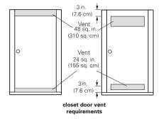
· Minimum vent opening for built-in installation is 31 ½ sq. in. (200 cm<sup>2</sup>).
