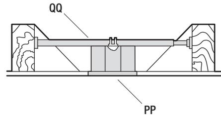
To hang your fan where there is an existing fixture but no ceiling joist, you may need an installation hanger bar (QQ) (not included) as shown above.
