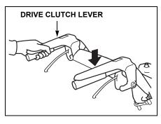
When both levers are depressed, the drive clutch lever locks the auger clutch lever down. This frees your right hand to operate the other snow blower controls. Releasing the drive clutch lever unlocks and releases the auger clutch lever.
