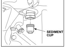
6. Empty the contents of the sediment cup into a suitable container. Clean the fuel sediment cup.
