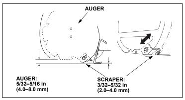
Adjust the scraper equally on both sides so that it remains parallel with the ground. Be sure to tighten the scraper bar bolts and nuts after making adjustments.
