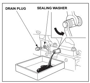
Allow the used oil to drain completely into an approved container, reinstall the drain plug with a new sealing washer, and then tighten it securely.
