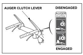
When both levers are depressed, the drive clutch lever locks the auger clutch lever down. Releasing the drive clutch lever then unlocks and releases the auger clutch lever.
