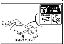
Pull both steering control levers at the same time to momentarily disengage the transmission. With the transmission disengaged, the snow blower is free to maneuver (push or pull) by hand with or without the engine running.
