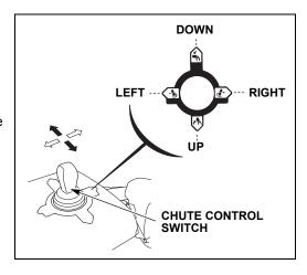
position when using the chute control switch.
