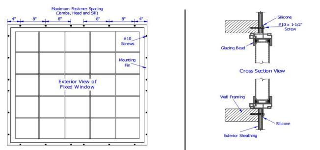
Note: We strongly recommend the use of flashing and/or flashing tapes and sill pans as stated in ASTM E 2112-01. However, due to variation in codes and building types, it is left up to the end user to determine the proper installation of these items.
