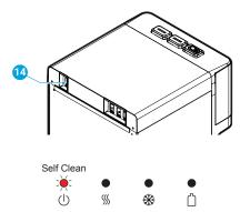
The power indicator light on the front of the dispenser will begin blinking, indicating the cleaning process is underway.
