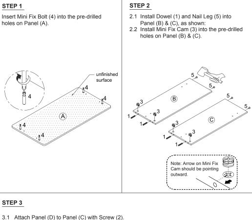
3.2 Attach Panel (B) to the assembled unit with Screw (2), as shown.
