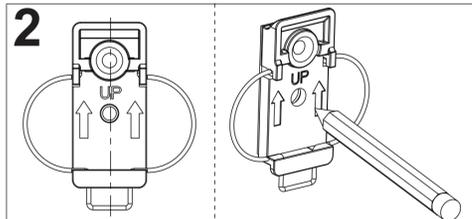
Position bracket on wall in desired location making sure that it is level. Mark (on the wall) location of fastener through bracket using a pencil.
