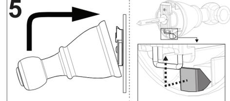
Hold the post at the base and place post over the bracket with the bottom edge against the wall. The catch at the bottom of the post should hook onto the spring at the bottom of the bracket. Then push the post upward and snap over the top edge of the bracket.
