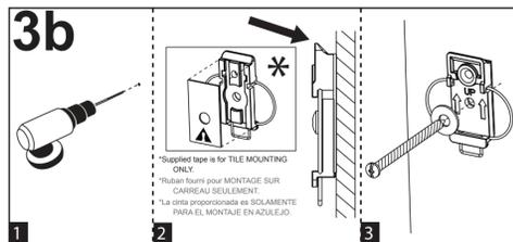
For stud installation in drywall: (1) drill 1/8" hole in centerpoint. (2) Place bracket with the spring on the bottom and the top edge angled toward the wall. (3) Insert #8 x 1-1/4" wood screw (not supplied), through the washer, into the center hole on the bracket and tighten screw until snug against wall. Do not over-tighten or press into the wall.
