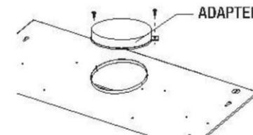
4. Measure the size of the outlet adapter relative to the cabinet and create an opening in the cabinet to let pass the outlet adapter and power cable. Make sure there is excess opening to accommodate electrical wires and hood exhaust. If you are installing the hood under the cabinet with a recessed bottom, it is advised to use a 4" wood fillers on both the sides.
