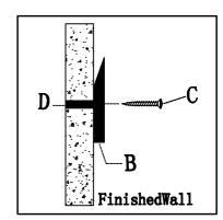
Pre-drill holes into the wall and attach part B to wall by using C and D.
