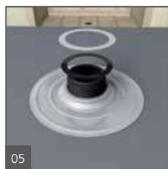
05 Turn the Fundo base upside down and apply the rubber and the fiber gasket.
