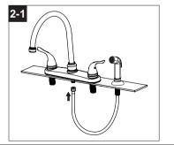
3. Connect the Water Supply Lines using a flexible braided supply line (3.1) (not included), connect the end with 1/2 in. female IPS to the tailpiece (3.2) of the faucet. Hand tighten. Do not overtighten. Install the other end of the supply line (3.1) to the shut-off valve or supply tube. NOTE: Consumer should follow the directions on the supply line and if you have any questions about proper installation of the supply line, consult the manufacturer of the supply line.
