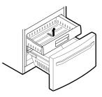
**4** Remove the Durabase basket from the rails. Remove the screws from the rails at both ends.
