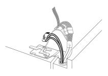
**5** Hold the water supply connection and gently push in the collet **(**) to connect the water supply line as shown. Insert the tube at least 5/8 inch (15 mm) into the connector. Insert the clip on the joint to fasten the tube in place.
