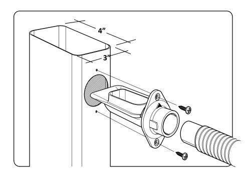
Be sure to remove the diverter regularly to clear leaves and debris that can collect above in the downspout.
