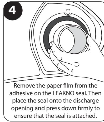
Remove the paper film from the adhesive on the LEAKNO seal. Then place the seal onto the discharge opening and press down firmly to ensure that the seal is attached.
