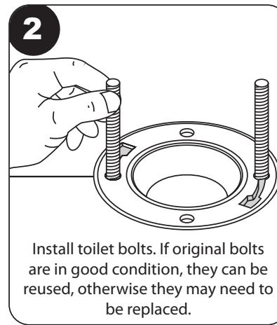
Install toilet bolts. If original bolts are in good condition, they can be reused, otherwise they may need to be replaced.
