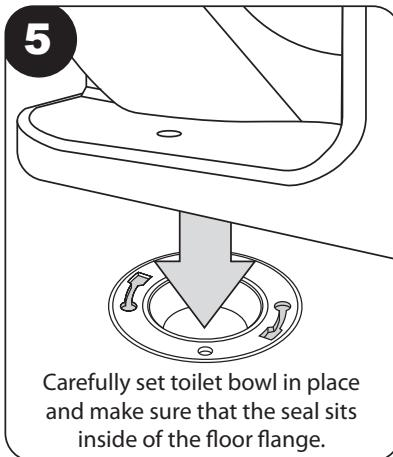
Carefully set toilet bowl in place and make sure that the seal sits inside of the floor flange.
