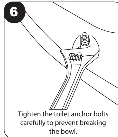
Tighten the toilet anchor bolts carefully to prevent breaking the bowl.
