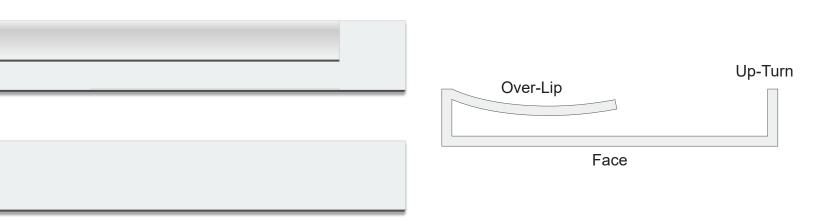
**EZ-On Main Covers** install on all your main beams and cross T's. They are cut to fit 2 ft. lengths of ceiling grid, have a tab at one end, and an over-lip and up-turn edge which allow them to slip on and click into place.
