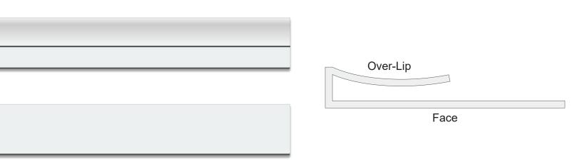
**EZ-On Wall Angle Covers** install along the edge of your ceiling, everywhere your grid touches a wall. They are cut to fit perimeter portions of ceiling grid, and have an over-lip along their length which holds them firmly in place.
