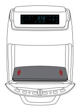
Slide Drip Tray into the oven's lowest position possible.
