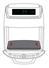
Slide Drip Tray into the oven's lowest postition possible.
