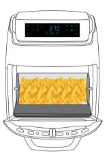
Slide Rolling Cage into the oven's grooves left side first.
