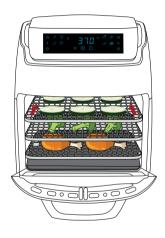
Place food on Grill Racks then slide into the Air Fryer Oven **Note:** This Air Fryer should only be used with the Drip Tray securely inside the appliance.
