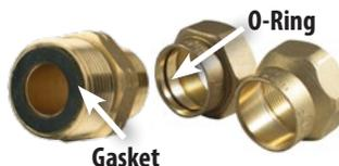
**Note:** DO NOT use sealing solution on parallel thread (gasket end) of fitting assembly. Gaskets cannot be reused, and must be replaced if fitting assembly is disassembled. Not all fittings include an o-ring and it is not part of the gas sealing mechanism.
