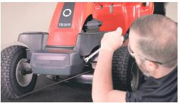
e. Replace the cotter pin to re-connect the steering rod.
