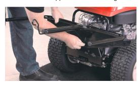
b. Connect to the center hole using wing knob and bolt.
