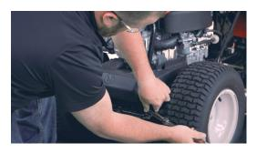
b. Assemble the mount to the frame and tighten using the 4 new bolts, using a 1/2" wrench.
