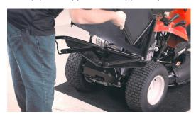
b. Using a 3/4" wrench, secure the two lock nuts.c. Add both bags.
