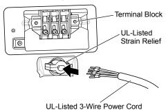
Attach the two hot leads (black and red) of the power cord to the outer terminal block screws. 5 Attach the neutral (white) wire to the center terminal block screw.
