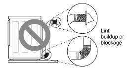
Make sure the ductwork is not crushed or restricted.
