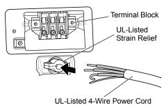
Transfer the dryer's ground wire from behind the green ground screw to the center screw of the terminal block.
