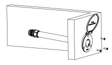
With the appropriate fitting threaded in, connect the hydrant to your plumbing system. If possible, add an expansion loop of PEX tubing. This allows the hydrant and fitting to be inspected and serviced from the exterior of the building, if ever needed. With copper, you may bracket the inlet against a stud, and then unscrew the entire hydrant body to access the internals.
