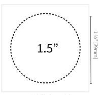
Use 1-1/2" drill bit for entry hole. Template included in hydrant box.
