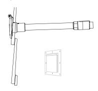
For the mounting holes, make sure to **insert the debris cover wedge behind** the hydrant faceplate. Secure to wall with #10 stainless screws.
