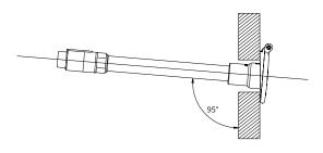
Drill the entry hole. 1-1/2" bit recommended.
