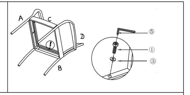
Attach Backrest Panel(D) to Seat Panel(C) using Bolts(1) and Washers(3) with Allen Key(5) as shown in the picture.
