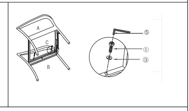
Attach Seat(C) to Right Armrest(B) using Bolts(①) and Washers(③) with Allen Key(⑤) as pictured.
