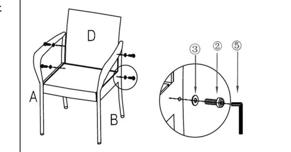
Attach Backrest Panel(D) to Left Armrest(A) and Right Armrest(B) using Bolts(2) and Washers(3) with AllenKey(5) as pictured.
