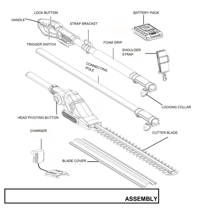
Aluminum Blade Support - Rubber Over Molded Handle - Hardened Steel Blades
