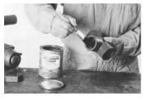
3. Put a second full even layer on the pipe/tube O.D.
