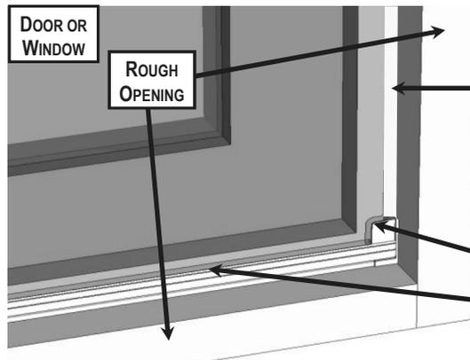
**NOTE \*2:** THE BEAD OF SEALANT SHOULD BE CONTINUOUS AND TOOLED FLAT. SOME SEALANTS MAY HAVE ADVERSE REACTION WITH CERTAIN SELF ADHERING FLASHING PRODUCTS. PLEASE VERIFY COMPATIBILITY WITH THE MANUFACTURER. THE FOAM AND THE SEALANT SHOULD OVERLAP AND HAVE AN AIR-TIGHT JOINT.
