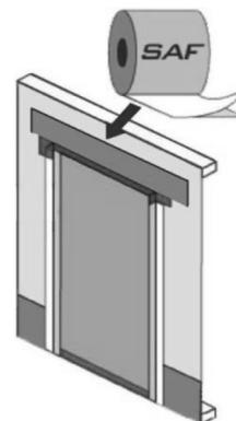
**IMPORTANT:** Seal the 1/8" gap behind window or door threshold with sealant and tool it flat. Back of the door/window casing should be grooved to accommodate for the sill pan.
