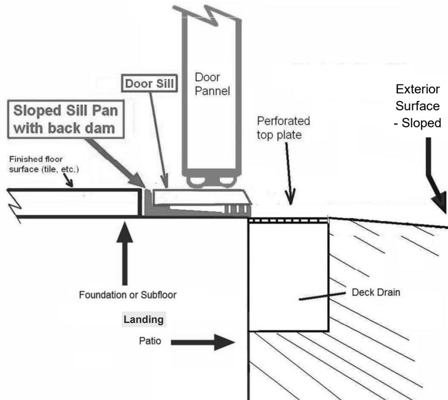
**Fig. 2 CONTINUOUS SLAB EXTERIOR DOOR DRAIN DETAIL**
