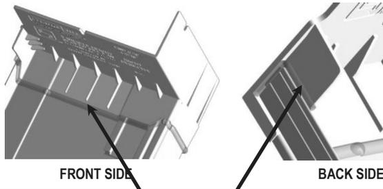
**DETAIL** REMOVE LABELS FROM CONTACT SURFACES. AS PART OF THE SILL PAN ASSEMBLY APPLY SEALANT ALONG THE EDGE OF END CAP. WITHOUT PROPER ASSEMBLY THE SILL PAN WILL LEAK. SURESILL™ IFS™ SHOULD BE INSTALLED AT THE SAME TIME A WINDOW OR DOOR IS BEING INSTALLED.
