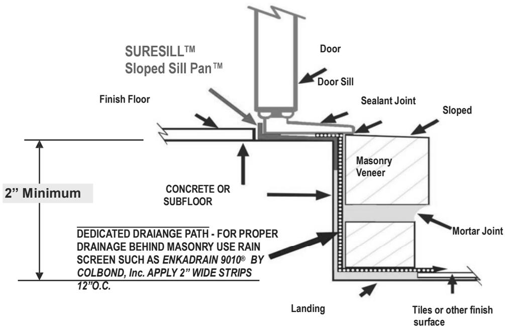
**Fig. 1 EXTERIOR DOOR WITH STEP-DOWN LANDING
