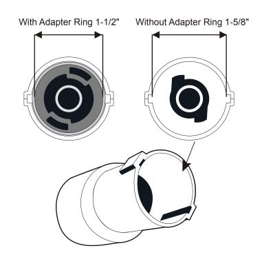
If the connection on the hose is slightly too small to fit the nozzle on your machine, try removing the preinserted inner adapter ring. Grip the outside of the connector firmly in one hand, while with the other, press and twist counter-clockwise from the inside.
