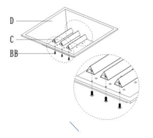
3.Put the 4pcs Steel Top(E) together, using 8pcs M6×12 Bolt(BB).
