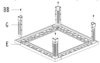
5. Attach the Side Panel(F) to the Leg(G), using 16pcs M6×12 Bolt(BB) .Tighten
