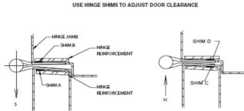
FIGURE 21 SHIMMING TO INCREASE CLEARANCE AT HINGE EDGE
