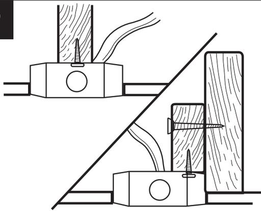
Use metal outlet box suitable for fan support (must support 35 lbs). Before attaching fan to outlet box, ensure the outlet box is securely fastened by at least two points to a structural ceiling member (a loose box will cause the fan to wobble).
