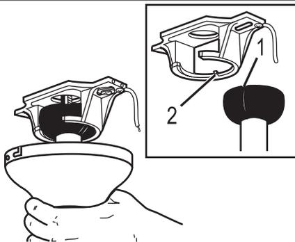
Carefully lift fan assembly onto mounting bracket. Rotate fan until notch on downrod ball (1) engages the ridge on the mounting bracket (2). This will allow for hands free wiring.
