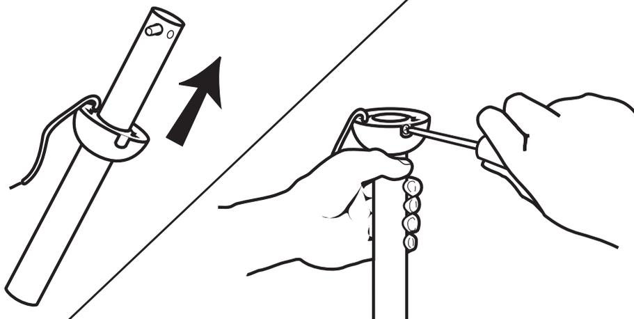
Re-install pin into extended downrod, and slide downrod ball up to the top of the downrod. Re-install set screw to secure ball to downrod. Note: Some extended downrods have a pre-drilled set-screw hole. If a pre-drilled hole is present in the extended downrod, tighten the set screw into the pre-drilled hole in the extended downrod. If no pre-drilled hole exists in the extended downrod, tighten the set screw against the downrod to secure the downrod ball.
