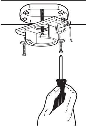
Install mounting bracket to outlet box in ceiling using the screws and washers provided with the outlet box.
