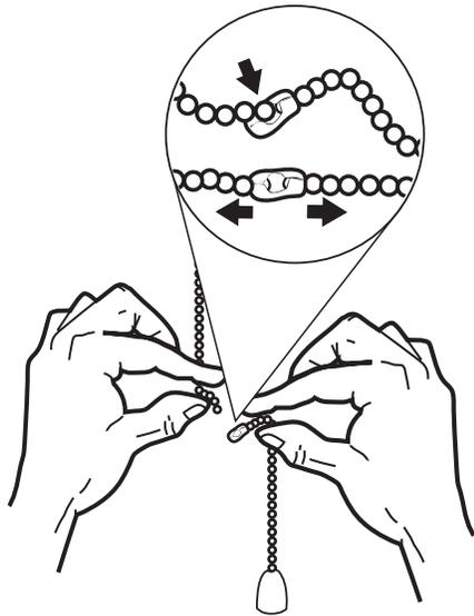
Assemble decorative fob and extension chains from hardware bag to fan pull chains by inserting end of chain into chain coupling. Confirm chains are held by lightly pulling both chains in coupling.
