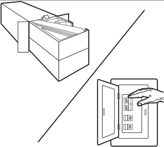
Unpack and inspect fan carefully to be certain all contents are included. Turn off power at fuse box to avoid possible electrical shock.
