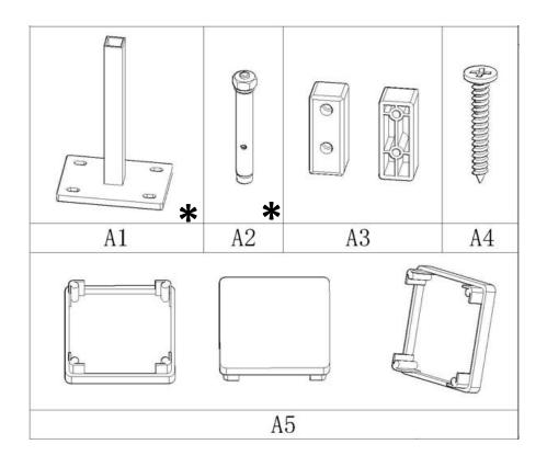
\* Components necessary for hard surface installation
