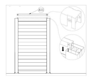
Finally, install the post caps (A5) to lock in the top cap rail and horizontal fence boards.
