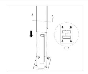
With the screws provided (A4), screw in the board stopper through both the post and fixing post support (Figure B-B).
