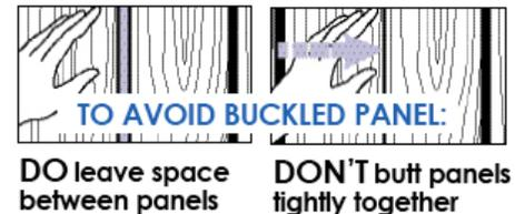
**Tileboard Installation Without a Divider Strip** For tileboard installation without divider strips, seal 1/8" space between panels with a high-quality silicone caulk. For a pleasing appearance, and a secure seal, carefully caulk around the tub. *Note: Panel adhesive must be dry before caulking. Wet adhesive may discolor caulk.*
