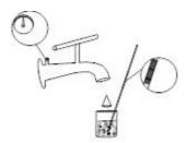
C. There should be a sewer. While working, some of the water will be discharged, so the sewer is necessary. Furthermore, the sewer must be kept unblocked.
