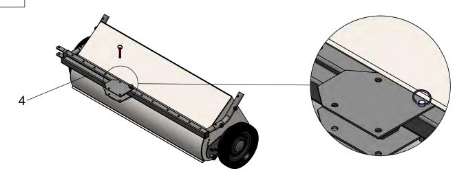
2 Replace pin in desired postion along Hitch Cross Tube
