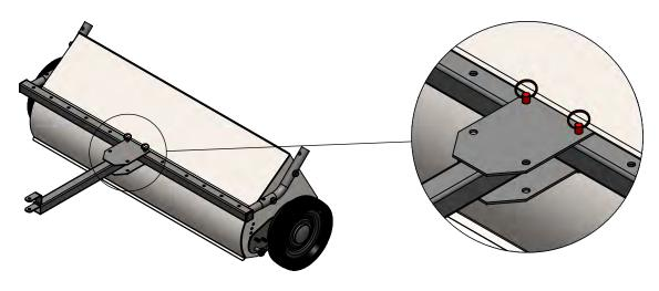
Attach Height Adjustment Handle Using a 9/16" Open End Box Wrench and
