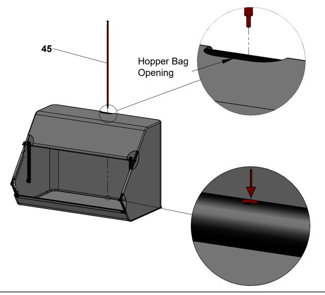
1 Lift Upper Center Frame Tube Over Tension Tube and Secure with Supplied Thumb Screw. Secure Hopper Bag around Top Frame Tubes with velcro tabs.
