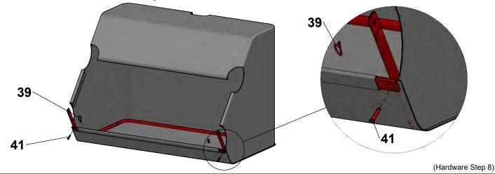
Place top frame assembly into Hopper Bag. Install Clevis Pins through Top Frame Tubes and Bottom Frame Tubes and secure with Hairpins.
