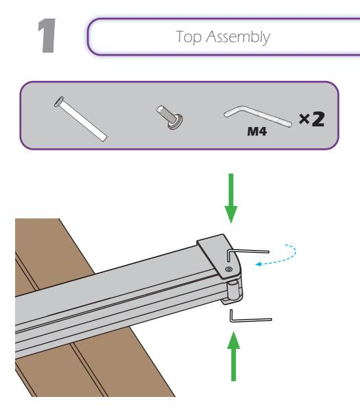
Press against the bolt with one wrench while turning the other wrench until secure.
