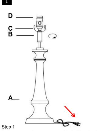
Pull power cord to connect the Neck (B) to the Base (A). Screw the Neck (B) onto the Lamp base (A) Be careful not to twist the power cord and tighten securely
