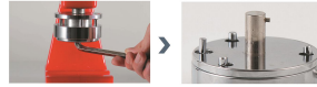
Figure 1: when the upper die is loose, the inner hexagon wrench can be used to tighten the mold. The standard is: 1.2.3 three points in a line
