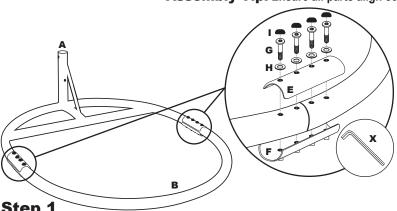
Align Base Back (A), Base Front (B), Top Base Connector (E), and Bottom Base Connector (F). Secure base parts using Bolt (G) and Washer (H). Tighten the hardware using the Small Hex Key (X). Place Bolt Cap (I) on top of the bolts.
