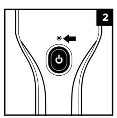
Plug the charging adapter into a wall outlet. The charging indicator liaht will blink. Light will go out when fully charged.
