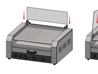
Insert No.7 and 8 into the front and side glass that have been installed and secure them with screws, as shown in the diagram.
