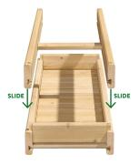
Slide the Top Layer over the ends of the **Dovetail Bottom Boards** to connect it with the Bottom Layer.
