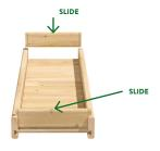
Once the floor is built - insert the last two **Dovetail Bottom Boards** into the **Routed Side Boards**.
