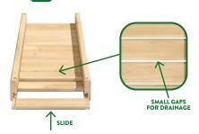
Slide thirteen **Dovetail Bottom Boards** into the routed edges of the **Routed Side Boards** to complete the floor. Make sure to leave small gaps between the **Dovetail Bottom Boards** for drainage.
