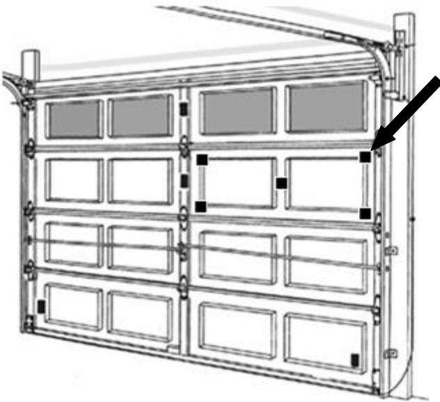
Begin by cleaning the surface of the inside door panels where the adhesive squares Stick'ems™) will be used to hold the radiant barrier panels in place.
