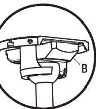
Receiver (B) correctly positioned in the mounting bracket.
