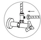
11. Connect the 78.7" metal hose we supplied to the open side of the T-valve.
