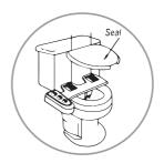
13. Place the toilet seat back on the toilet over the bidet and secure the bolts down so that the seat and bidet attachment are stable.
