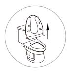
Remove the existing toilet seat by locating the bolts and nuts, typically under a plastic cover, and removing them first.
