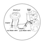
14. Connect the hoses from step 6 & 10 to the corresponding hot and cold bidet water connections underneath the handle of the BB-270.
