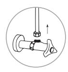
8. Disconnect the water hose from your sink's hot water supply valve.
