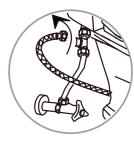
6. Connect the 25.5" metal hose we supplied to the open side of the T-Valve.
