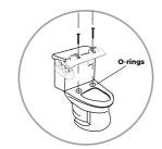
12. Place the bidet on the toilet with the mounting brackets over the bolt holes. Center the bidet on the toilet so that you can see the bolt holes through the mounting brackets of the bidet. Place the Protective O-rings under the mounting bracket to protect and secure the bidet on the toilet.
