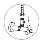
10. Attach the water supply hose that comes from the water shut off to the top of the T-valve.
