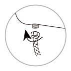
3. Disconnect the water hose from underneath the toilet tank.
