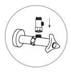
9. Connect the 3/8" T-valve to the hot water supply valve where you just removed your water hose. Make sure the runner washer is included into the connection.
