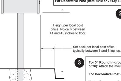
For 3" Round In-ground Post (item 7507 or 7516) or Standard In-ground Post (item 5525): Pour the concrete (at least 1 cubic foot recommended) completely around the post, making sure the post and mailbox are level and correctly positioned according to your local post office.
