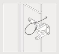
B Mount latch cover (C) on post above latch (B).
