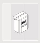
Open Yardlock, move lever to original position, and install rubber cover.
