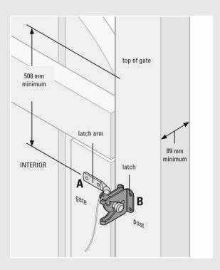
B Secure latch assembly with supplied screws.
