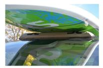
1. Lay pads across top of car roof w/ flat side down.
