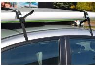
7. Tie knot with the remaining loose strap (very close to the buckle to keep strap from slipping in buckle). Tie/wrap remaining strap to roof rack or pinch in window to prevent flapping in the wind.
