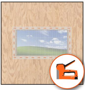
2. Staple along the top with approximately 1 inch spacing, keeping the Kwikmesh smooth and flat. Continue with the sides and finish with the bottom.
