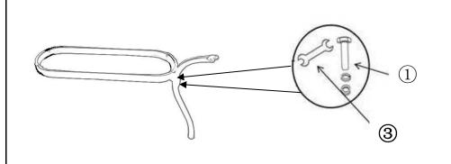
Loosely attach the Central Support Ring(C) to Table Legs(B) using washers, Spring Washers, and Hex Bolts(①), with the Spanner(③).
