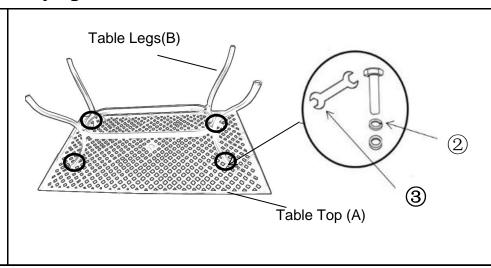
Lay the Table Top(A), top facedown onto a flat, soft, clean surface. Attach the Table Legs(B) to the the Table Top(A) using Washers, Spring Washers, and Nuts(②) with the Spanner(③).
