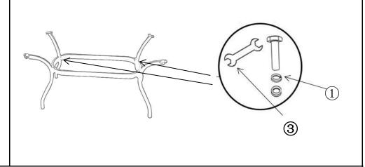
Repeat step 2, attaching the remaining 3 legs to the Central Round Support Ring(C)
