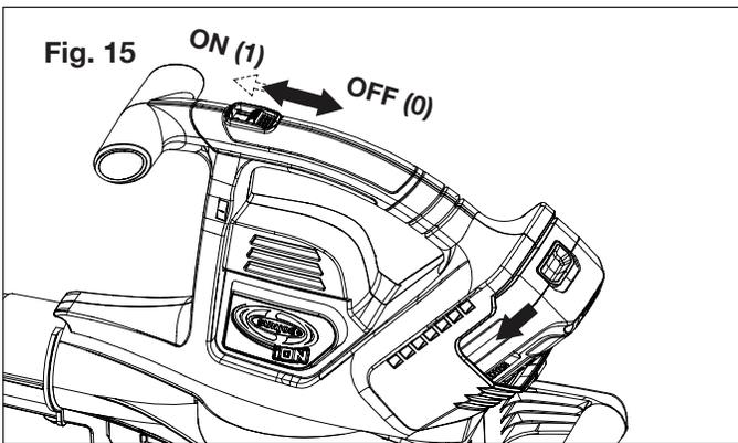
3. To stop the unit, slide the ON/OFF switch to the OFF position (0) (Fig. 15).
