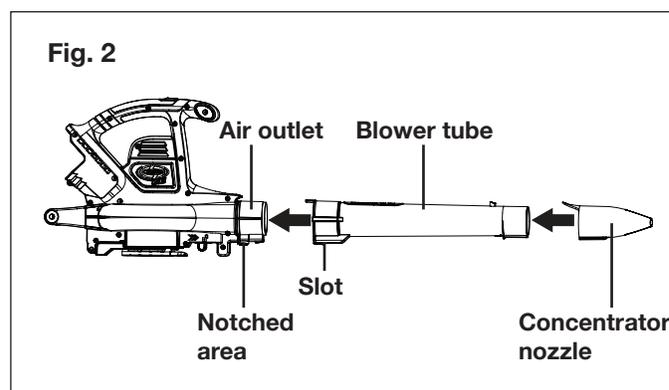
4. To remove the blower tube, turn the ON/OFF power switch to the OFF (0) position and remove the battery.
