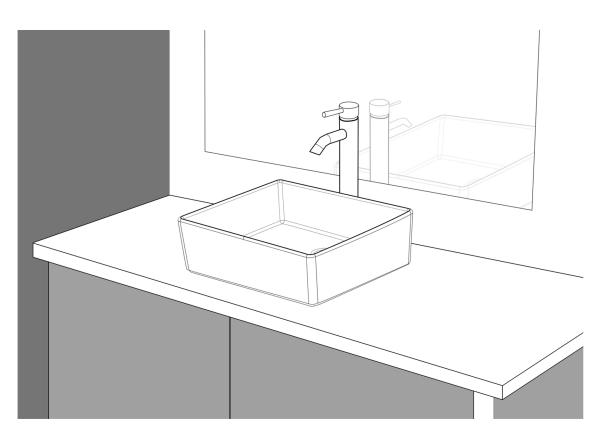
Step#2: Once the position is confirmed, mark the center of the drain hole and set aside the vessel sink. Draw a 3 inch diameter circle around the center of the drain hole. Use a jigsaw or a power tool to cut the opening on the countertop.
