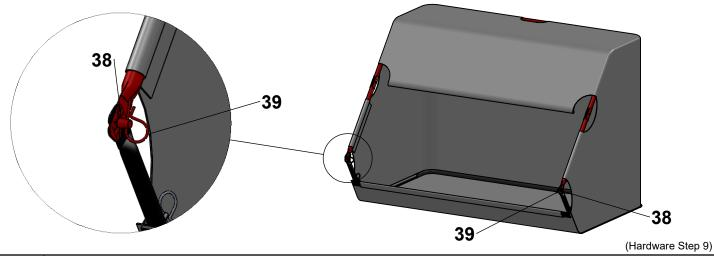
From one side, slide Pivot Rod through Top Frame Tube, Connecting Tube and pocket of Hopper Bag. After Passing all the way through the Hopper Bag pocket, thread Pivot Rod through other Connecting Tube and Top Frame Tube. Now Secure both protruding ends with a Washer and Hairpin Cotter.
