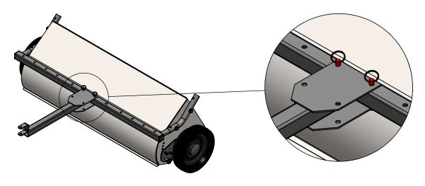
3 Attach Height Adjustment Handle Using a 9/16" Open End Box Wrench
