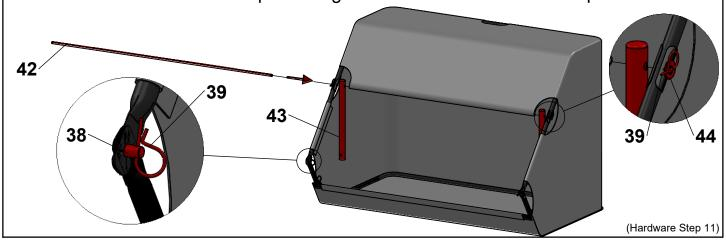
Hold Hopper Bag open and carefully insert Tension Tube through opening in top of hopper and into hole in Bottom Center Frame Tube.
